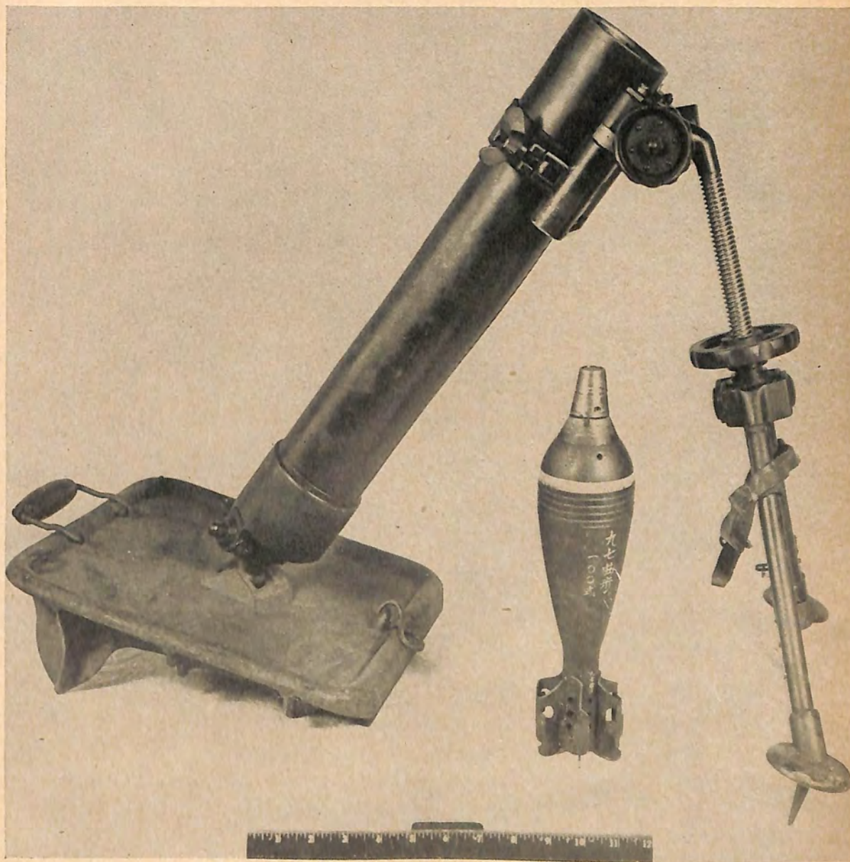
Figure 192. Model 99 (1939) 81-mm mortar and standard projectile.
